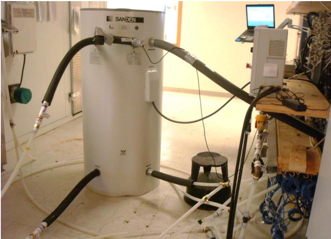
Figure 3 shows a schematic of the general test setup. Cascade Engineering installed an instrumentation package to measure the required points specified by the DOE test standard, as well as additional points to gain further insight into HPWH operation.
